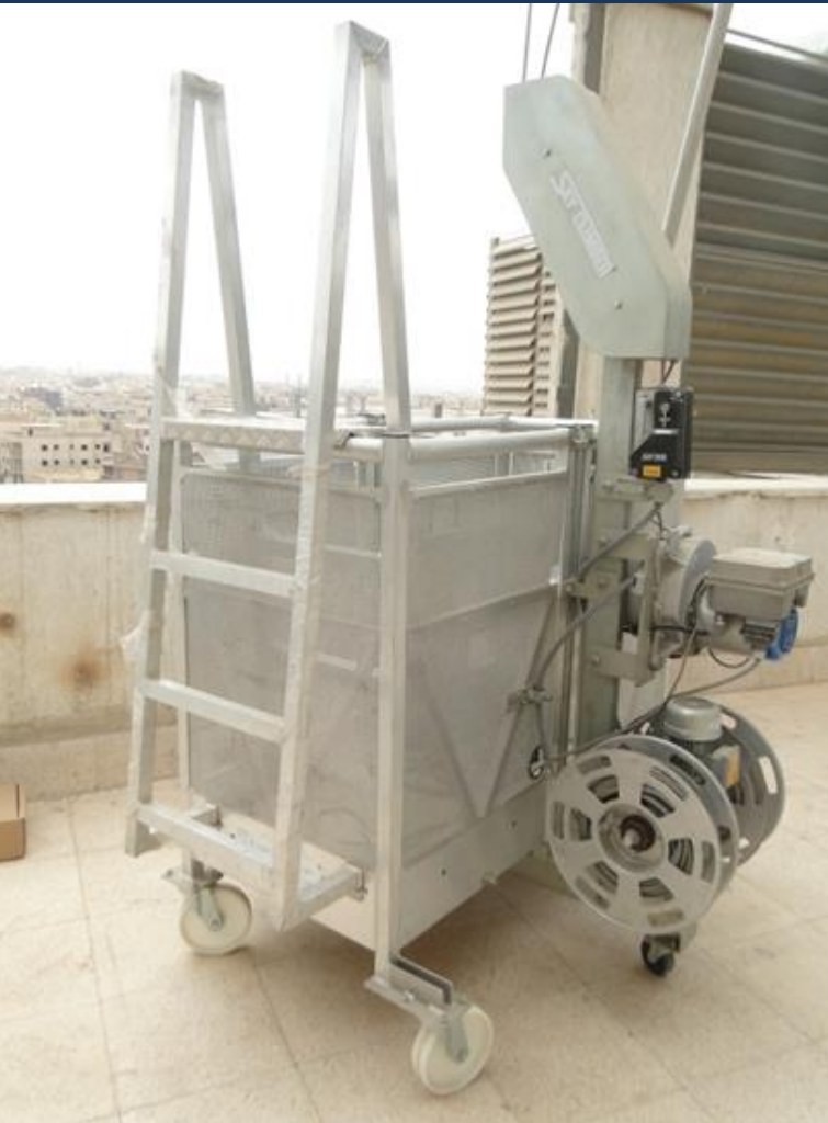
1,5 m mesh cladded Light Weight Cage for permanent installation with CX500 hoist, Sky Lock, wire winder and access ladder
